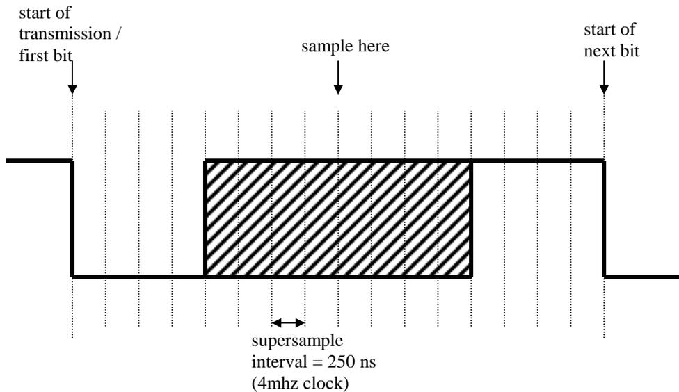
There is a tricky timing issue in the receiving stage that arises because the board clock is not exactly the same frequency as the controller clock. This may cause the FSM to become unsynchronized with the controller signal.
