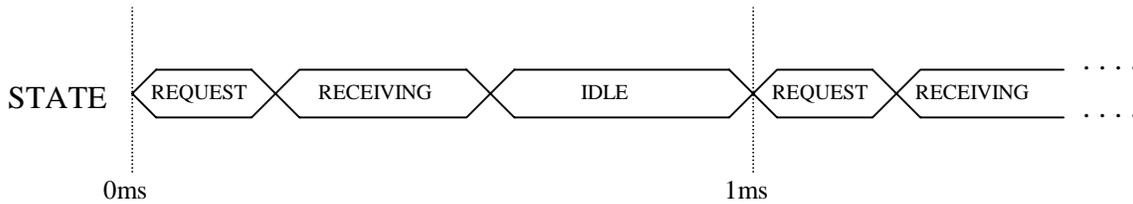
For sending the request signal, it is necessary to count  $1\mu\text{s}$  intervals, since each bit consists of four  $1\mu\text{s}$  sections. This can be done by counting four 4mhz clock cycles.
