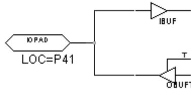
Notice that the OBUFT is a tri-state buffer. Be aware that the control signal "T" is active low, so the output buffer will be enabled (i.e. signals will be output to the pad) when T = 0. When the IOPAD is not being used to output signals, the OBUFT should be turned off (to Z state).
