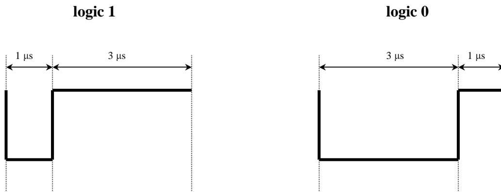
To receive the controller button information, the request byte 0x01 (hexadecimal) must first be sent to the controller. Also, a stop bit (logic 1) must be sent as a 9<sup>th</sup> bit of the transmission. Viewed on the oscilloscope, the request waveform should look like this:
