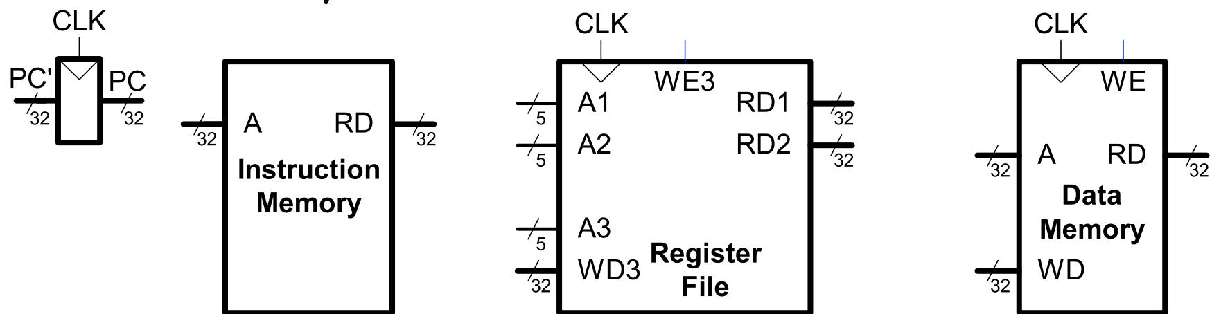
Note: for these state elements, clock is used for write but not for read (asynchronous read, synchronous write).
