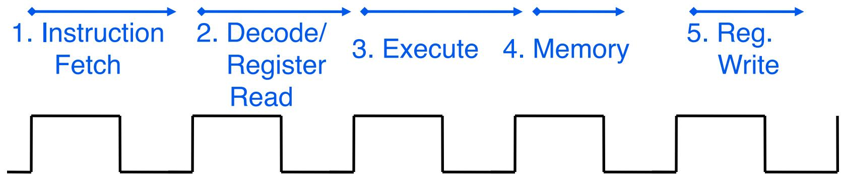
Several significant advantages over single cycle execution: Unused stages in a particular instruction can be skipped OR instructions can be pipelined (overlapped).
