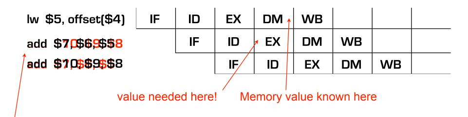
"Architected load delay slot" on MIPS allows compiler to deal with the delay. Note, regfile still needs to be bypassed.
