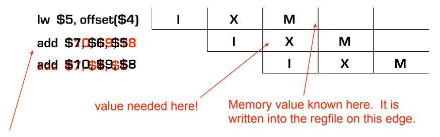
"Architected load delay slot" on MIPS allows compiler to deal with the delay. No regfile bypassing needed here assuming regfile "write before read".
