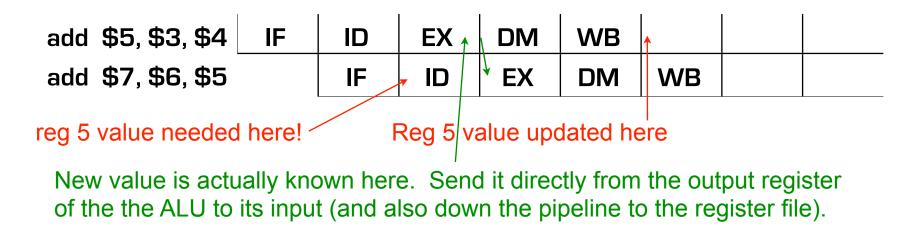
Logic must be added to detect when such a hazard exists and control multiplexors to forward correct value to ALU. No alternative except to stall pipeline (thus hurting performance).
