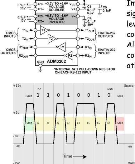
Implements standard signaling voltage levels for serial communication. Allows FPGA board to communicate with any other RS-232 device.
