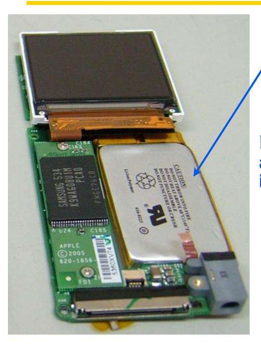
1.2 W-hour battery: Can supply 1.2 watts of power for 1 hour.
