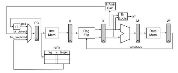
The BTB has been added in the Fetch Stage. The BTB is indexed by the PC register in the Fetch Stage. Branch address calculation has been moved back to the Execute Stage.
