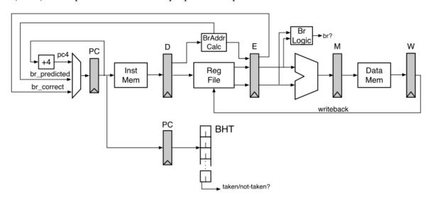
The BHT has been added in the Decode Stage. The BHT is indexed by the PC register in the Decode Stage. Branch address calculation has been moved to the Decode Stage. This allows the processor to redirect the PC if the BHT predicts "Taken".
