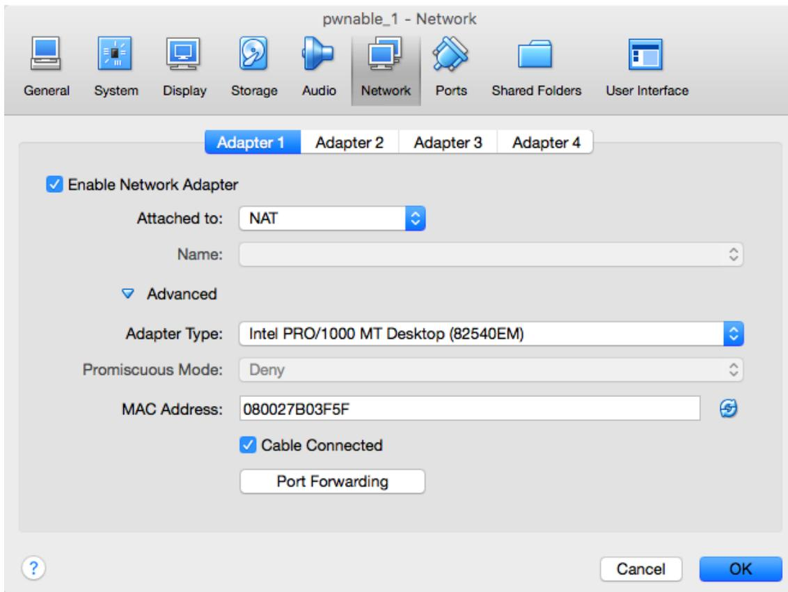
Click the **Port Forwarding** button and ensure that you have a rule to forward port 22, for SSHing to the machine, to port 2222 on your host. Also make sure that **Cable Connected** checkbox is checked.
