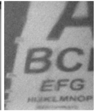
Figure 6. Reflections in two other tea pots, taken from a distance of 5m. The 18pt font is readable from the reflection in the left picture, and almost readable in the right picture.
