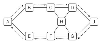
The machine A has initiated a TCP connection to machine J. As it turns out, all packets from A to J happen to follow the path indicated by the right-facing dotted arrows, and all packets from J to A happen to follow the path indicated by the left-facing dotted arrows. Machines A and J use modern TCP software and do not have any special defenses against attack.
