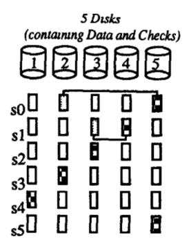
Note: Due to the large size of disks in practice, RAID V is no longer used in practice, because it is too likely that a second disk will fail while the first is recovering. RAID VI is usually combined with other error recovery techniques in practice.
