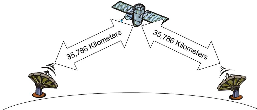
**Problem 4a[4pts]:** Suppose that you have a dedicated satellite connection between two points on the earth. The satellite will be in a geostationary orbit (at an altitude of 35,786 km). Assume that we will be using TCP over this connection. Assume that the satellite forwards all bits after a 100ms latency (fully pipelined, since there is no routing in the satellite). Also assume that we can use “jumbo TCP frames” with an MTU of 9000 bytes.
