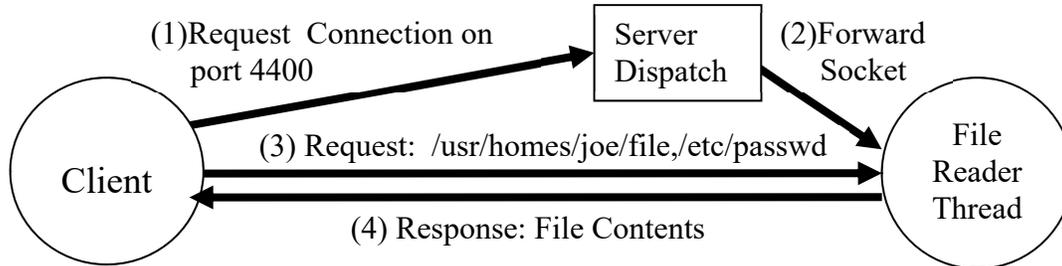
Here, the client sets up a TCP socket connection with the server on port 4400, then sends one or more file names separated by “,” and/or newline characters. Finally, the file reader thread sends the contents of the specified file(s). The client terminates by sending a blank line.
