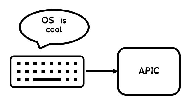
Device sends electric signal over interrupt request line (IRQ) to interrupt controller
