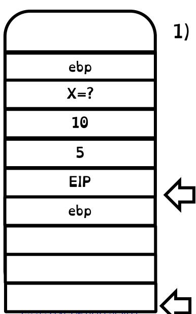
1) Save frame pointer and set to stack pointer
