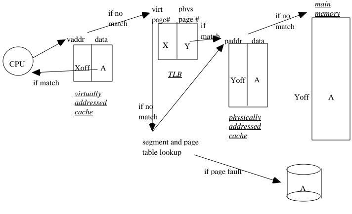
If between translation box and memory, called a "physically addressed cache". Could also put a cache between CPU and translation box: "virtually addressed cache".
