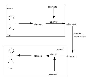
From cipher text, can't derive plain text (decode) without password. From plain text and cipher text, can't derive password!
