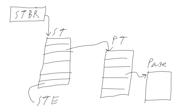
Combination of segments and pages. We put valid bit, dirty bit in page table. protection bits in segment table, or in page table, but usually in segment table since all pages share the same protection. Each segment has a bounds field to hold its size
