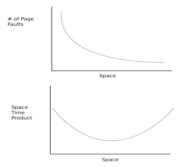
\*SPT is the integral of the amount of space used by the program over time.  $\int space(t)dt$ \*Discrete time:  $\sum m(i)(1+f(i)PFT)$  PFT is page fault time.
