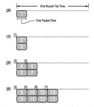
The horizontal direction is time. The continuous time line has been chopped into oneround-trip-time pieces stacked vertically with increasing time going down the page. The grey, numbered boxes are packets. The white numbered boxes are the corresponding acks.
