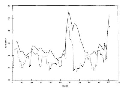
Same data as above but the solid line shows a retransmit timer computed according to the algorithm in appendix A.
