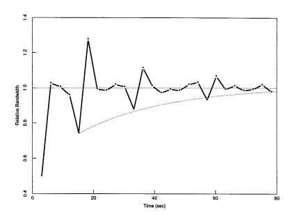
Because of the five second averaging time (needed to smooth out the spikes in the old TCP data), the congestion avoidance window policy is difficult to make out in figures 10 and 11. Here we show effective throughput (data acked) for TCPs with congestion control, averaged over a three second interval.
