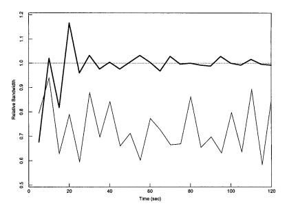
Figure 10 showed the old TCPs were using 25% more than the bottleneck link bandwidth. Thus, once the bottleneck queue filled, 25% of the the senders' packets were being discarded. If the discards, and only the discards, were retransmitted, the senders would have received the full 25 KBps link bandwidth (i.e., their behavior would have been antisocial but not self-destructive). But fig. 8 noted that around 25% of the link bandwidth was unaccounted for.
