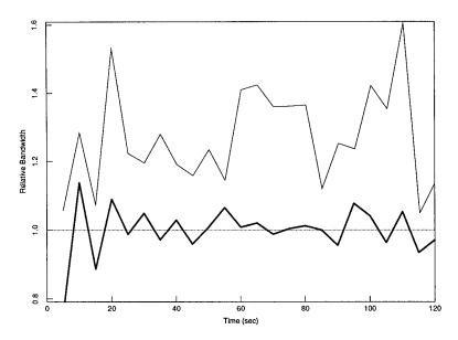
The thin line shows the total bandwidth used by the four senders without congestion avoidance (fig. 8), averaged over 5 second intervals and normalized to the 25 KBps link bandwidth. Note that the senders send, on the average, 25% more than will fit in the wire.
