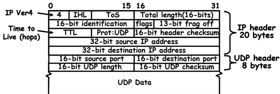
We will use UDP/IP for our implementation. The packet format is shown above. UDP/IP communication is *connectionless*. To communicate on a given port, an application simply *binds* a socket to that port, after which it can immediately begin sending and receiving messages on that
