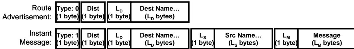
Remember that the UDP/IP header also contains information about which IP address and port was the source of the message.
