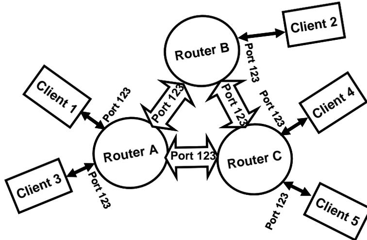
This problem will investigate the construction of a peer-to-peer communication network built. We will utilize instant messaging as our application on top of this network. As you see by the above figure, clients connect with individual routers. Messages transit from a source client to a destination client via one or more hops through a router.
