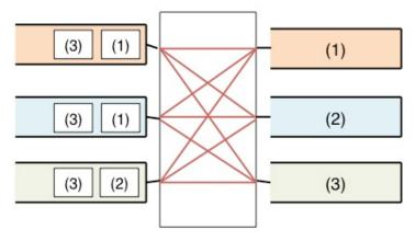
The router to the left receives has three input/output ports and a switched interconnect as described in class ("3<sup>rd</sup> generation" routers).
