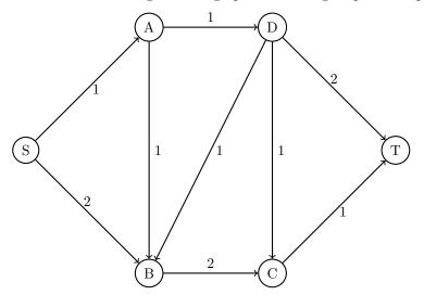
In the first step of Maximum-Flow algorithm, we increase the flow along  $S \to A \to D \to B \to C \to T$  by one unit.
