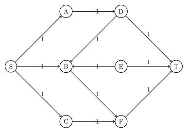
In the first step of Maximum-Flow algorithm, we increase the flow along  $S \to A \to D \to B \to F \to T$  by one unit.
