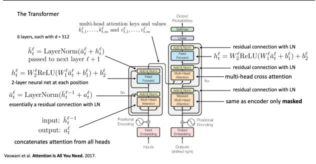
Figure 1: The diagram of the Transformer architecture.
