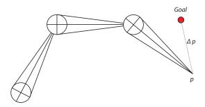
Figure 3: 3-jointed arm with goal position
