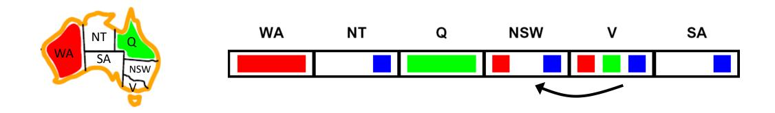
Arc V to NSW is consistent: for every x in the tail there is some y in the head which could be assigned without violating a constraint
