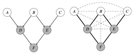
Which of the dotted line edges do we need to add so that the resulting MRF can encode the same conditional independence relations among the variables A, B, C as the Bayes Net above?
