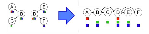
• Perform a **backwards pass** of arc consistency. Iterating from i = n down to i = 2, enforce arc consistency for all arcs  $Parent(X_i) \longrightarrow X_i$ . For the linearized CSP from above, this domain pruning will eliminate a few values, leaving us with the following:
