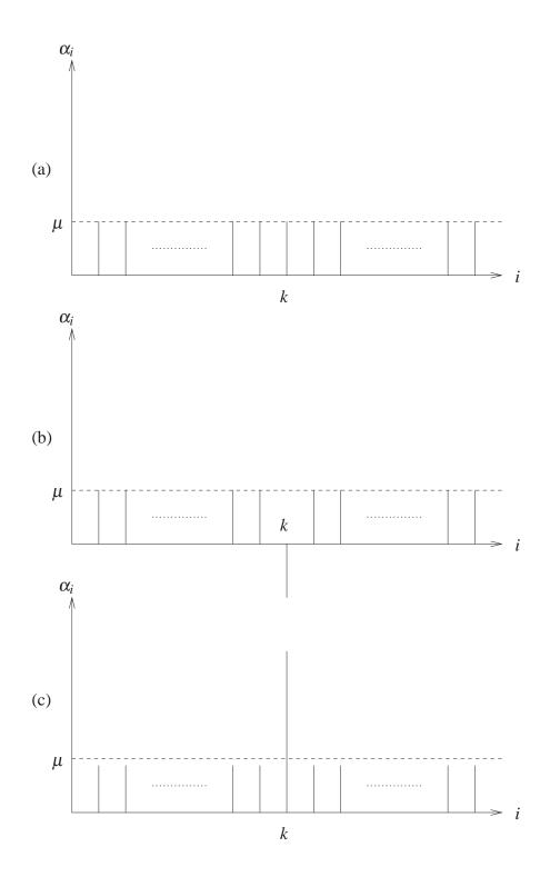
Figure 0.1: The first three steps of Grover's algorithm. We start with a uniform superposition of all basis vectors in (a). In (b), we have used the function f to invert the phase of  $\alpha_k$ . After running the diffusion operator D, we amplify  $\alpha_k$  while decreasing all other amplitudes.
