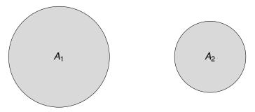
$A_1$  is twice the area of  $A_2$ , and we will assume that the diameter  $(d_1)$  and focal length (f) of  $A_1$  is 1, so the F-number would be 1. Let us further assume that the focal length of the lenses are the same. To figure out the F-number of  $A_2$ , we need to determine how much smaller the diameter is compared to that of  $A_1$ . Lets do the math!
