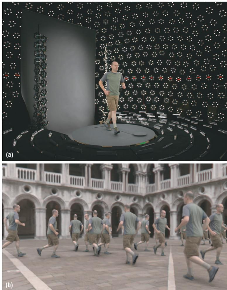
**Figure 6.** The Light Stage 6 performance relighting system. (a) A running subject is recorded in Light Stage 6, an 8-meter sphere that captures dynamic subjects under a wide array of viewing and lighting directions. (b) Several instances of the runner are rendered into a photographed environment, each with its viewpoint and illumination chosen to be consistent with the virtual scene.
