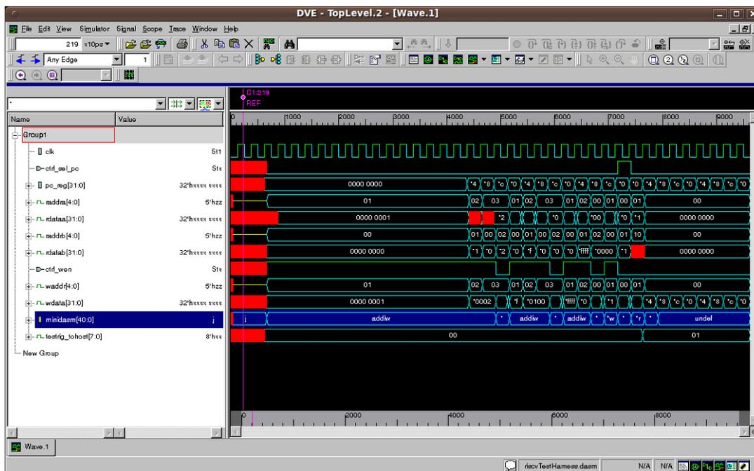
Figure 5: Waveforms for unpipelined RISC-V v1 processor executing `riscv-v1.addiw`
