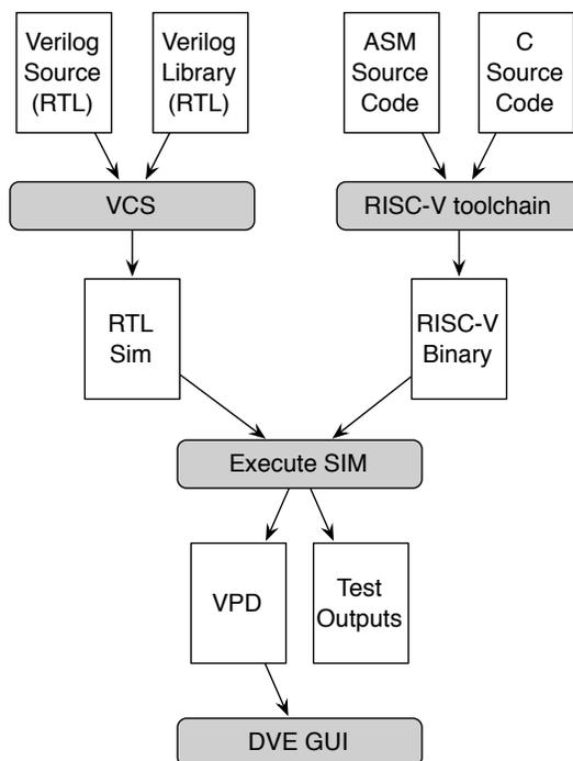
Figure 1: VCS Toolflow and RISC-V Assembler Toolchain
