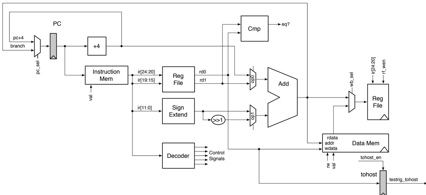
Figure 2: Block diagram for Unpipelined RISC-V v1 Processor
