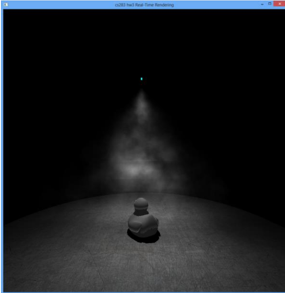
Figure 5. Interpolated deep shadow maps. The layer boundaries are not as visible, but some artifacting can still be seen. 64 shadowmap layers.
