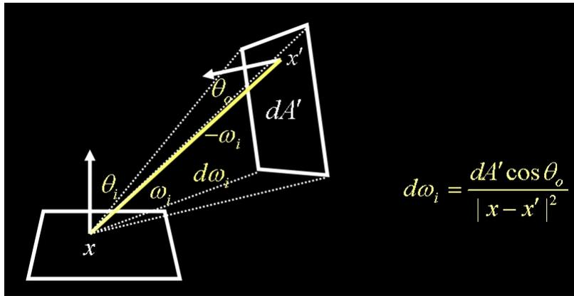
Figure 5: Deriving the surface parameterization of the rendering equation.
