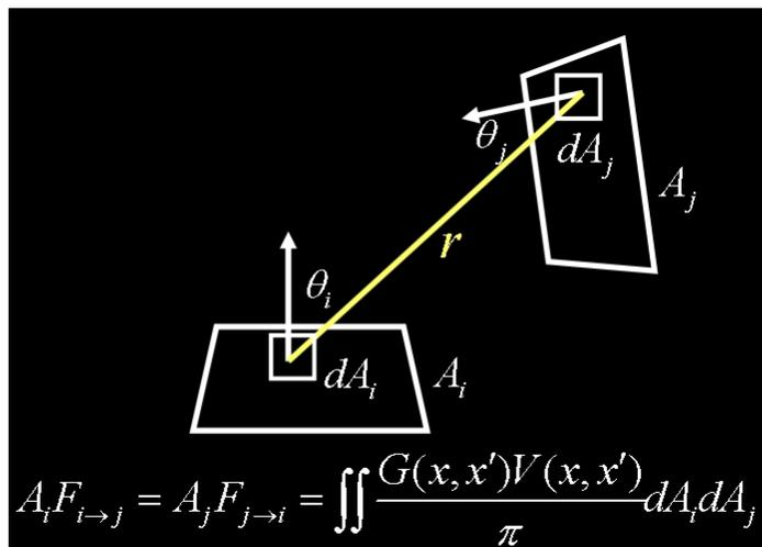
Figure 6: Deriving form factors for the radiosity equation.
