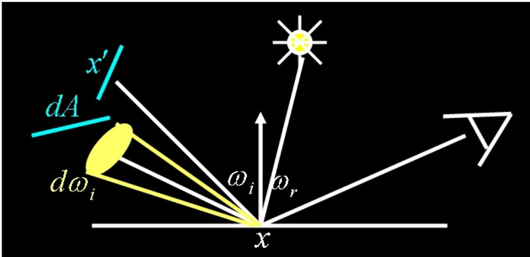
Figure 3: Local geometry for the rendering equation.
