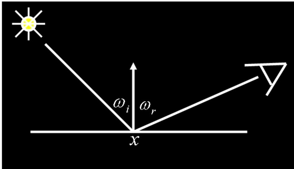
Figure 2: Local geometry for the reflectance equation.
