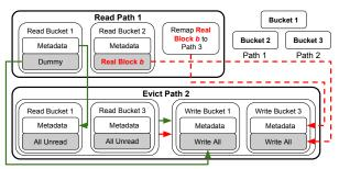
Figure 7: Multilevel Pipelining for a read of path 1 and an evict path of path 2 executing in parallel. Solid green lines represent physical dependencies and dashed red lines represent data dependencies. Inner blocks represent nested operations
