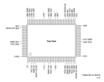
Figure 25: PQ100 PQFP with 100 Leads, .65 mm Lead Pitch
