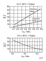
Figure 13: Typical Output V/I Characteristics
