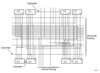
Figure 8: Example Routing Detail
