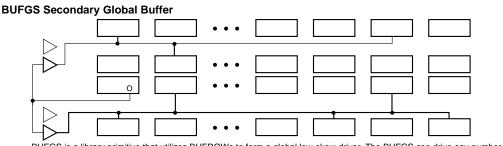
BUFGS is a library primitive that utilizes BUFROWs to form a global low-skew driver. The BUFGS can drive any number of CLCs, since it uses a BUFROW to drive the CLCs in each row. If there are no driven CLCs in a row, then no BUFROW is used in that row. Like the BUFROW, the BUFGS can be driven by a CLC (shown above) or by an IBUF input buffer.
