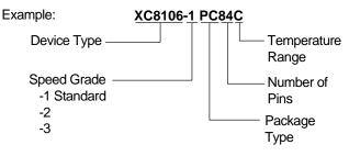
Note: Each Speed Grade can operate at 5 V or 3.3 V
