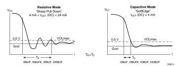
Figure 12: Output Slew Rate Options
