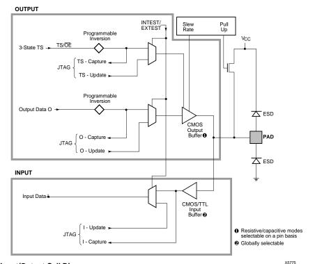
Figure 11: Input/Output Cell Diagram
