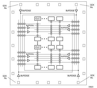
Figure 9: XC8100 Buffer Configurations
