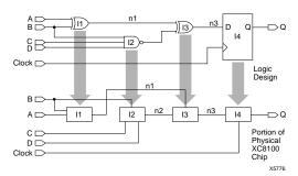
Figure 2: TrueMap<sup>™</sup> Logic Mappings
