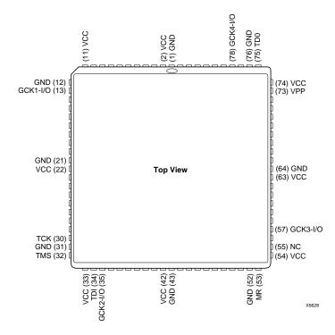
Figure 24: PC84 PLCC with 84 Leads, 50 mil Lead Pitch
