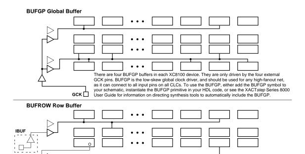
There are four BUFROW buffers for every two rows of CLCs, two on each end. The BUFROW can only drive the inputs of CLCs in the two rows adjacent to the BUFROW. Any CLC in any row can drive the input to the BUFROW. Using the BUFROWs as individual clock drivers allows more than four different clocks in a design. The above figure shows two BUFROW examples; one BUFROW driven by an IBUF input buffer, the other BUFROW driven by an internal CLC.
