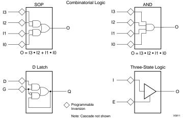
Figure 5: Programmable Cell
