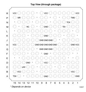
Figure 27: BG225 Plastic Ball Grid Array with 225 PbSn Balls, 15 x 15 Array, 1.50 mm Lead Pitch
