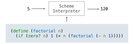
An interpreter can be parameterized to simulate any machine
