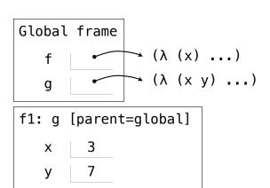
The way in which names are looked up in Scheme and Python is called lexical scope (or static scope) [You can see what names are in scope by inspecting the definition]
