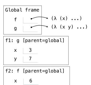
The way in which names are looked up in Scheme and Python is called lexical scope (or static scope) [You can see what names are in scope by inspecting the definition]
