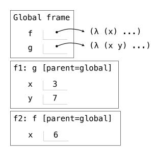
The way in which names are looked up in Scheme and Python is called lexical scope (or static scope) [You can see what names are in scope by inspecting the definition]
