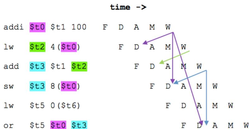
Without forwarding, the register values become available in the write-back phase, and are needed in the decode phase.
