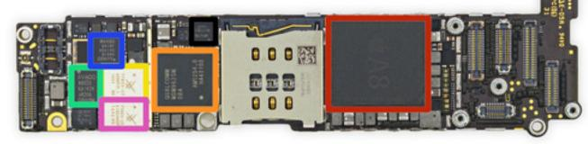
The A8 is manufactured on a 20 nm process by TSMC. It contains 2 billion transistors. Its physical size is 89 mm<sup>2</sup>. <sup>1</sup> It has 1 GB of LPDDR3 RAM included in the package. It is dual core, and has a frequency of 1.38 GHz.
