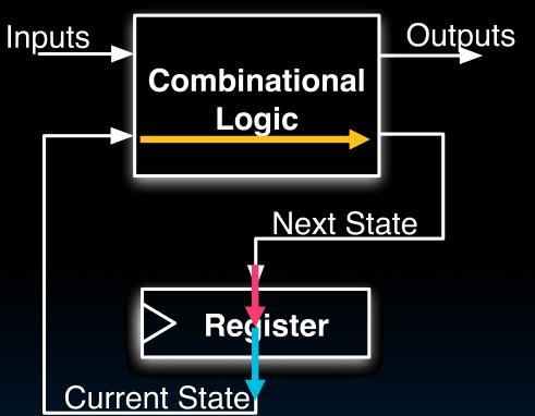
Max Delay = CLK-to-Q Delay + CL Delay + Setup Time
