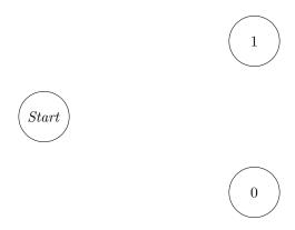
Draw an FSM that will output a 1 if it recognizes the regex pattern  $\{10+1\}$ . (That is, if the input forms a pattern of a 1, followed by one or more 0s, followed by a 1.)
