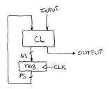
On each clock cycle the CL block looks at the input value and the present state and produces the bit pattern for the next state and generates an output of 0 or 1. On the rising edge of the clock the new state value gets captured by the register and the process starts again.
