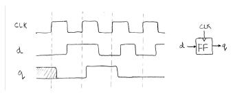
On each positive clock edge \_\_\_\_\_, the q output is changed to the current value of the d input.
