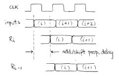
Notice that the maximum clock frequency (minimum clock period) is limited by the propagation delay of the add/shift operation. If we try to make the clock period too short, then the add/shift logic would not have sufficient time to generate its output and the output register would capture an incorrect value.
