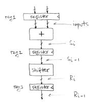
On each cycle, data moves from the output of reg1 through the adder to the input of reg2, or moves from the output of reg2 through the shifter to the input of reg3. Since the data no longer needs to move through both blocks on each cycle, the clock frequency can be increased. See the waveforms below:
