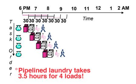
CS 61C L29 CPU Pipelining (9)
