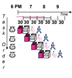
Suppose new Washer takes 20 minutes, new Stasher takes 20 minutes. How much faster is pipeline?
