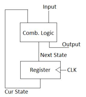
The register holds the current state (encoded as a particular combination of bits), and the combinational logic block maps from {current state, input} to {next state, output}.
