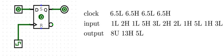
You'll notice that the value of the output in the diagram above doesn't change immediately after the rising edge of the clock. Clock cycle time must be small enough that inputs to registers don't change within the hold time and large enough to account for clk-to-q times, setup times, and combinational logic delays.
