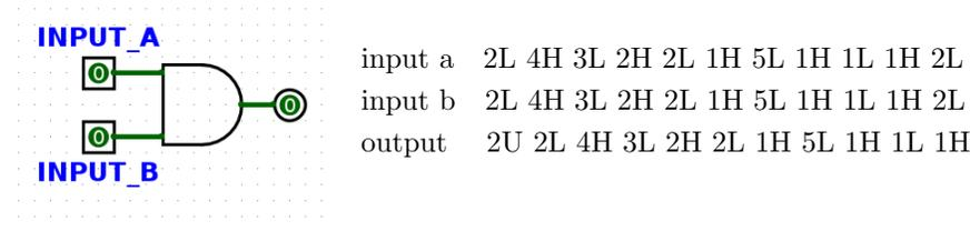
Where U, L, and H refer to an undefined, low (0), or high (1) signal respectively, for some number of nanoseconds.
