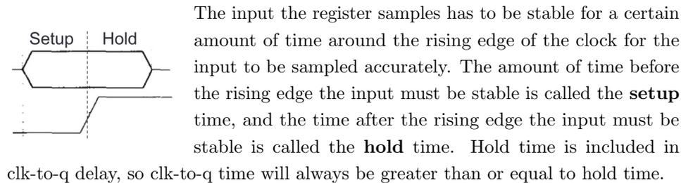
For the following register circuit, assume **setup** of 2.5ps, **hold** time of 1.5ps, and a **clk-to-q** time of 1.5ps. The clock signal has a period of 13ps.
