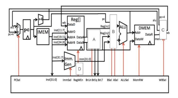
(a) Consider the following modifications to the branch comparator inputs. Which configuration will allow this instruction to execute correctly without breaking the execution of other instructions in our instruction set?
