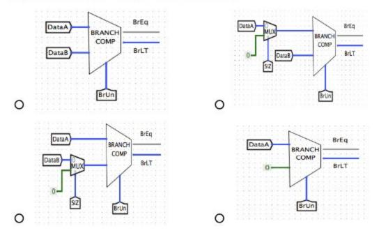
(b) Consider the following modifications to the ALU inputs. Which configuration will allow this instruction to execute correctly without breaking the execution of other instructions in our instruction set? Select the configuration that requires minimum modifications to the original datapath. Notice in the bottom left choice BSel is unused.
