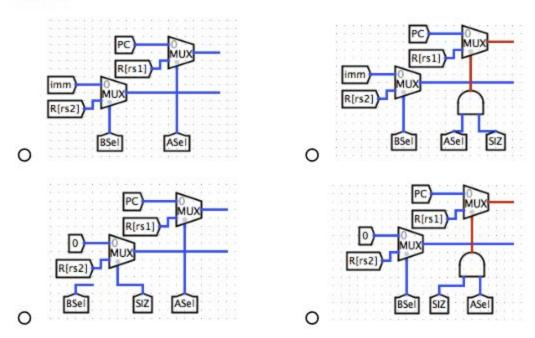
(c) Consider the following modifications to the WB mux inputs. Which configuration will allow this instruction to execute correctly without breaking the execution of other instructions in our instruction set? Select the configuration that requires minimum modifications to the original datapath.
