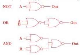
Using these three gates and applying the sum of products technique we can compute any boolean function.
