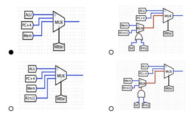
Solution: Similar to the previous question, we do not need to make a modification to the datapath and should therefore select option A. We know our ALU is emitting the value stored in register rs2. Because the standard datapath already allows us to write back the output of our ALU (and because write-back by default writes to our specified destination register rd), the value in rs2 can be written back to rd by setting our existing control bit WBSel to ALU. Again, no modifications are required.
