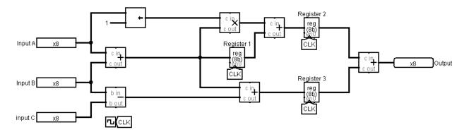
Figure 2: Non-pipelined circuit
