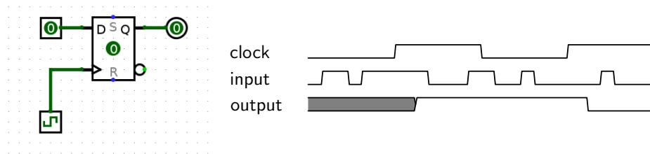
You'll notice that the value of the output in the diagram above doesn't change immediately after the rising edge of the clock. Clock cycle time must be small enough that inputs to registers don't change within the hold time and large enough to account for clk-to-q times, setup times, and combinational logic delays.
