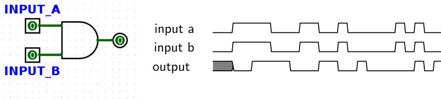
You should notice that the output of this AND gate always changes 2ps after its inputs change.
