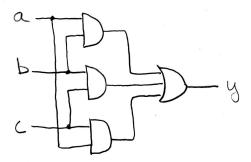
If we want to understand the operation of the circuit for any particular set of input values, we can manually apply the values to the circuit, propagating the correct value to the output of each logic gate, and finally to the output. In this case, applying an input pattern of 001 would result in an output of 0, whereas an input pattern of 101 would result in a 1 at the output. We could fully characterize the function of this circuit by trying all possible input patterns to generate a true-table.
