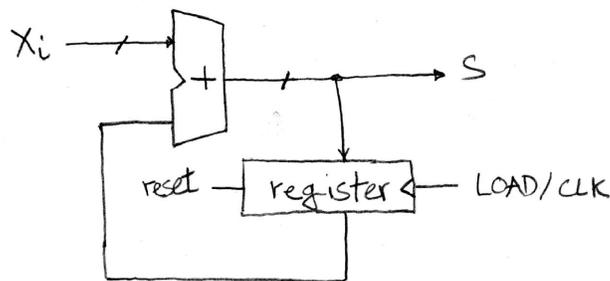
The register holds the current value of  $S$  while the next one is being formed. After we are happy with the next  $S$ , we load it into the register and apply the new  $X$  value, then wait for a new  $S$  to appear at the output of the adder. The process is repeated for all  $n$   $X$  values.
