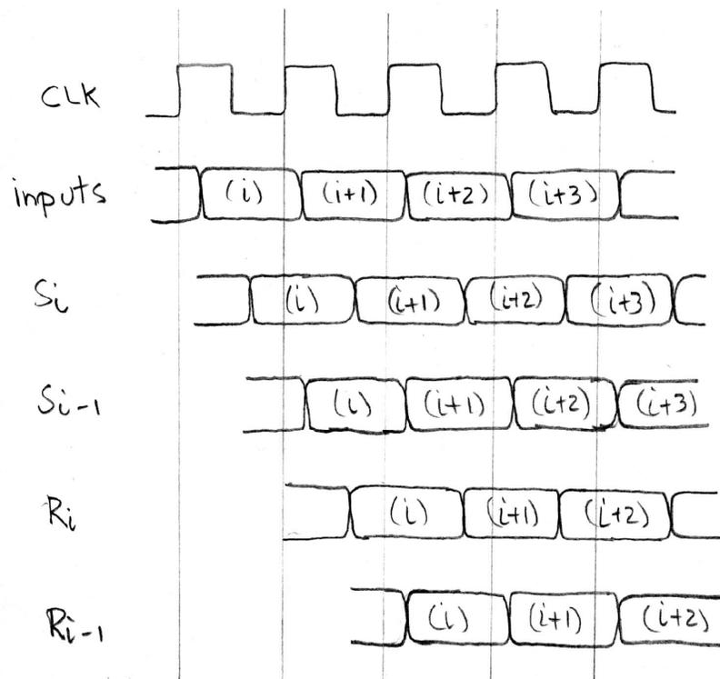
An interesting thing about this new circuit is that after the data moves through the adder and gets captured in reg2, on the next cycle when the data moves into the shifter, new data can simultaneously move into the adder, because it is free. Therefore new data values can be fed into the circuit on each clock cycle.
