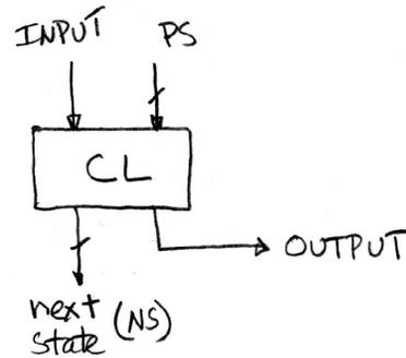
Given that we want to force a state transition on each clock cycle (remember inputs bits are being applied one per clock cycle), we will put the combinational logic block in a loop with the state register as shown below:
