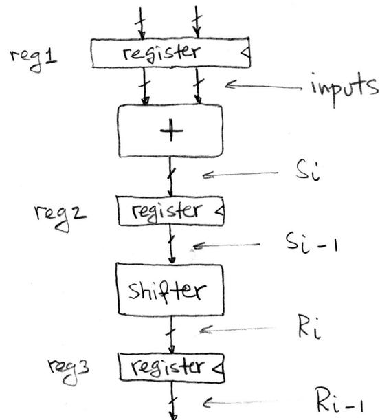
On each cycle, data moves from the output of reg1 through the adder to the input of reg2, or moves from the output of reg2 through the shifter to the input of reg3. Since no longer does the data need to move through both blocks on each cycle, the clock frequency can be increased. See the waveforms below:
