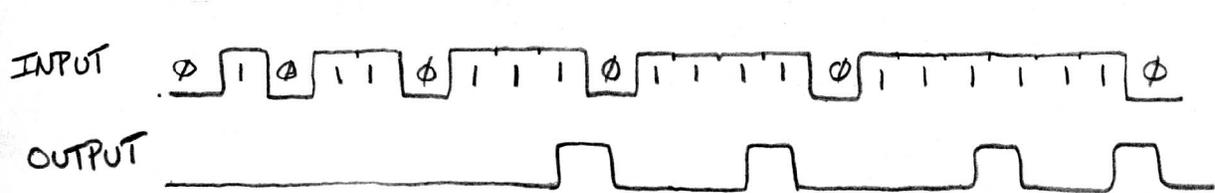
We begin the design of the FSM by drawing the state diagram. The  $S_0$  state is the state the machine is in when it begins counting 1s.  $S_1$  means the machine has seen one 1 and  $S_2$  means the machine has just seen the second 1. In  $S_2$  if the machine sees another 1 then the output is changed to a 1 and the machine goes back to  $S_0$ . If in  $S_2$  the machine sees a 0, then the output remains at 0 and the machine returns back to  $S_0$ .
