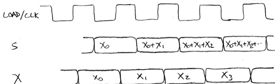
Later we will discuss the detailed timing of the operations in the accumulator circuit, but first we need to look at the detailed operation of the register.
