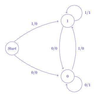
5.3 Draw an FSM that will output a 1 if it recognizes the regex pattern {10+1}. (That is, if the input forms a pattern of a 1, followed by one or more 0s, followed by a 1.)
