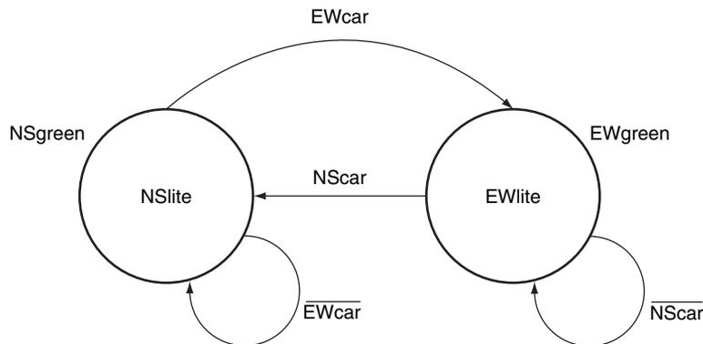
**FIGURE C.10.2** The graphical representation of the two-state traffic light controller. We simplified the logic functions on the state transitions. For example, the transition from NSgreen to EWgreen in the next-state table is  $(\overline{\text{NScar}} \cdot \text{EWcar}) + (\text{NScar} \cdot \text{EWcar})$ , which is equivalent to EWcar.
